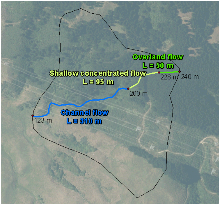
Figure 4-4 Time of concentration component parts
