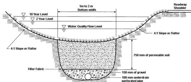
passes through the invert of the swale, through a loam soil, then geotextile fabric and gravel prior to discharge through a 100 mm perforated pipe.
