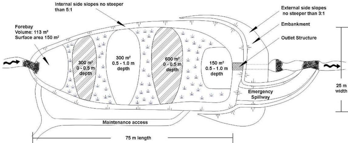
As the forebay elevation is considered part of the wetland surface area, the areas detailed in the banded bathymetric design have been reduced proportionally to account for the forebay area. If the individual areas are added together the total recommended levels are achieved.
