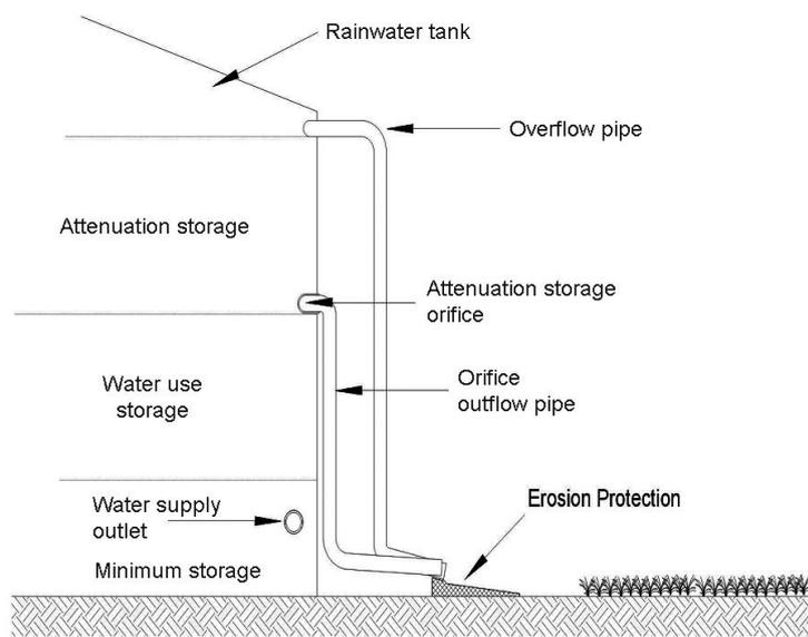
Normally, detention volumes would be determined by the difference in volumes of the pre-and post-development 2- or 10-year storms. Using the 10-year storm as the worst-case scenario, the 10-year 1-hour rainfall should be used for storage purposes. The amount of detention storage required depends on the daily water use by the commercial or industrial operation. Storage volumes related to roof area are shown in Figure 7-28.
