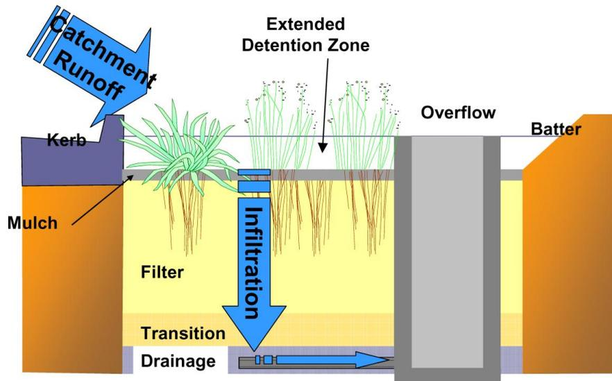
Rain garden design, as shown in Figure 7-10 differs only slightly from sand filter design. Where sand filtration relies on water quality treatment via passage of stormwater through sand, rain gardens incorporate plants and soils for removal of contaminants. A downside of the use of plants and soils rather than sand is a reduction in the permeability rate. This results in rain gardens being larger in surface area than sand filters.
