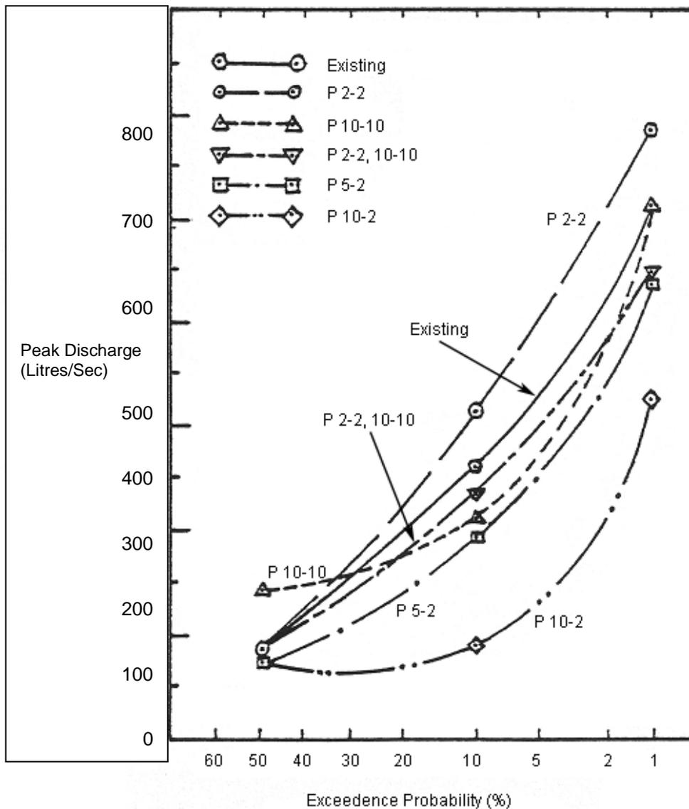
In the above figure, P stands for policy while the first number after the P stands for the post-development storm frequency while the second number stands for the pre-development storm frequency. A P 2-2 reflects a policy where the post-development peak discharge for the 2-year storm cannot exceed the pre-development peak discharge for the 2-year storm. A P 5-2 policy means that the post-development 5-year peak discharge cannot exceed the 2-year pre-development peak discharge.
