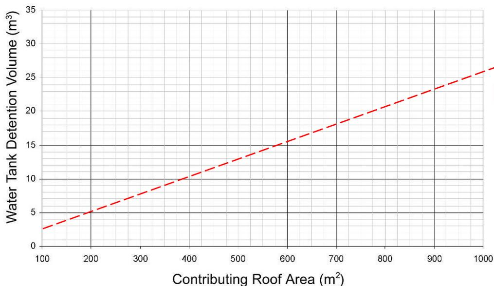
The required orifice size is a function of the storage volume and the depth of water above the orifice. This depends on the tank size selected to accommodate the water use and attenuation volume. The tank diameter, in conjunction with the attenuation
