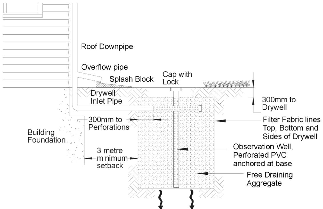
Dry wells function in a similar fashion with the excavated subgrade being filled with stone and relying upon the void spaces to provide for stormwater storage until the runoff infiltrates into the soil.
