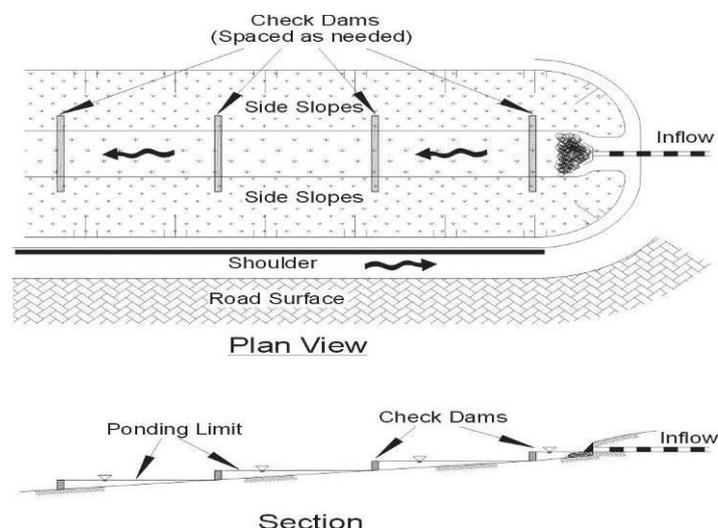
the normal approach is to accept that the average flow through the swale does take nine minutes. There will be areas in the upper part of the swale that may exceed the required residence time so the average is appropriate in light of the benefits that swales provide.
