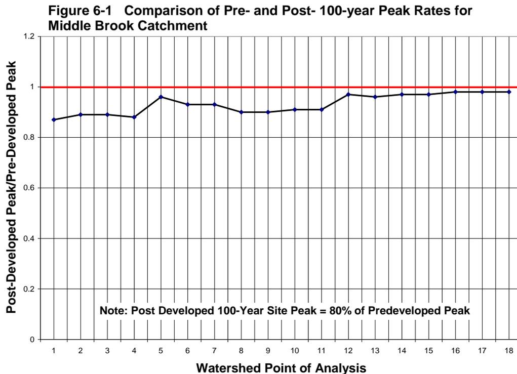
An examination of this comparison shows that, under this level of peak rate control, post-developed runoff rates are less than pre-developed for the entire storm. This increased time period offers greater opportunity for this and other post-developed site hydrographs with similar levels of control to combine downstream in such a way as to produce a total downstream peak that is no greater than the pre-developed peak at that location.
